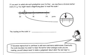
Fig. 1. An extract from the workbook dealing with reading analog scales.
