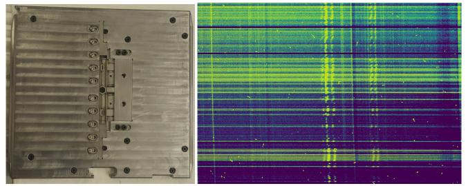
Figure: Left: The fully assembled SMI-200 instrument. Right: Spectra of a star-forming galaxy through several fibers of SMI (each individual horizontal trace is spectra from a fiber). The vertically misaligned zig zag blobs are Hydrogen-alpha (brightest), doubly ionized Nitrogen and Sulphur emission lines.
