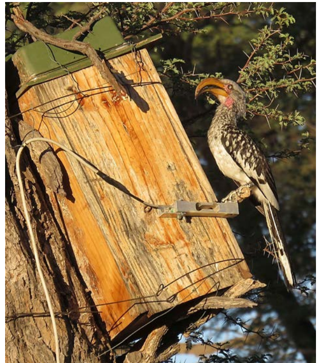
A male Southern Yellow-billed Hornbill sits on a perch attached to a load-cell at the entrance to his nest-box. PhD student Tanja van de Ven used these load-cell "perch scales" to monitor the body mass of breeding birds (Photo: Dean Portelli).
