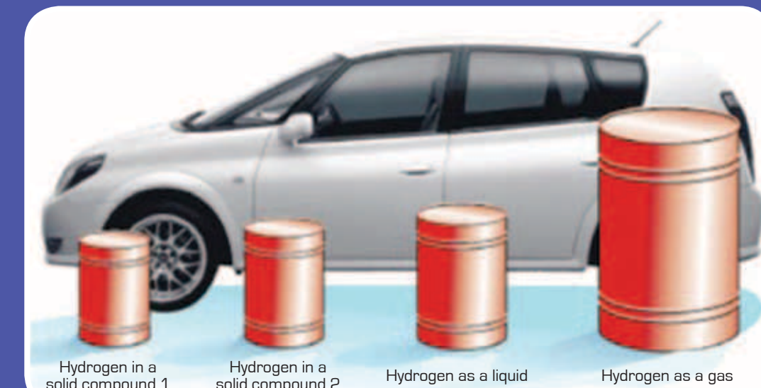
Sizes of tanks that would be needed for hydrogen in different forms
