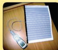
M. Harting, UCT silicon nanoparticles mixed in an ink, allows solar cells to be printed. This means you can charge your cell phone wherever you are.
