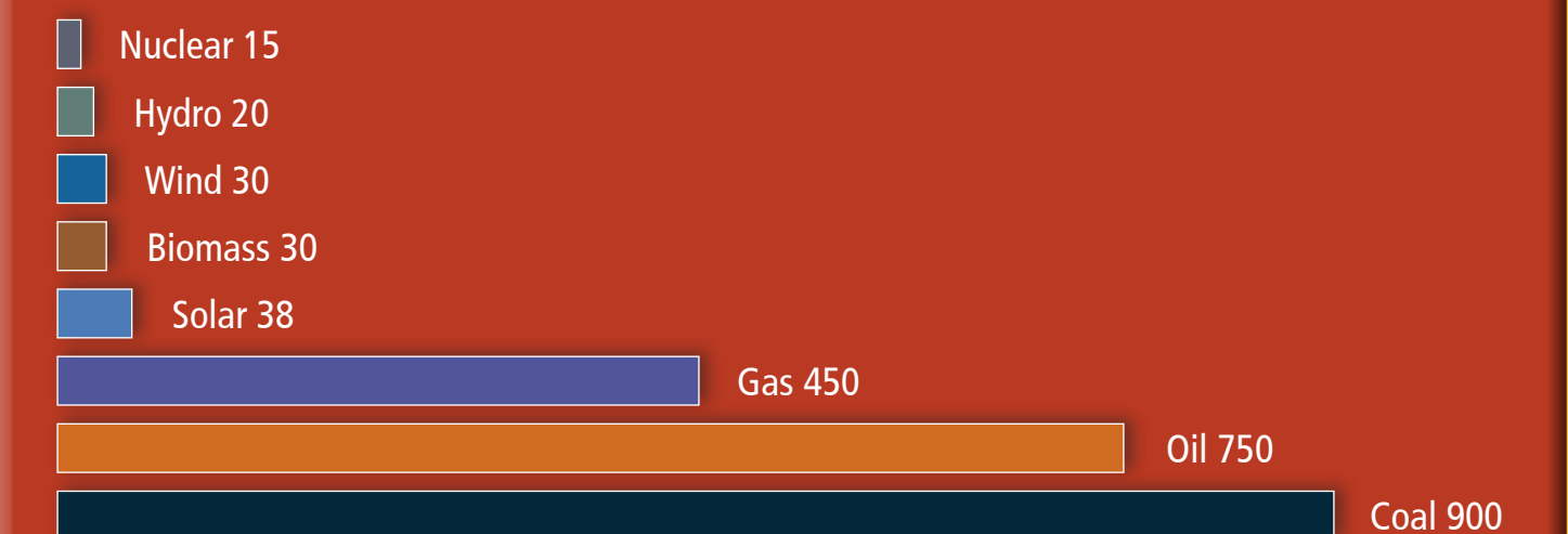
CO 2 EMISSIONS FROM DIFFERENT ENERGY SOURCES (grams of CO 2 equivalent per kilowatt hour)
