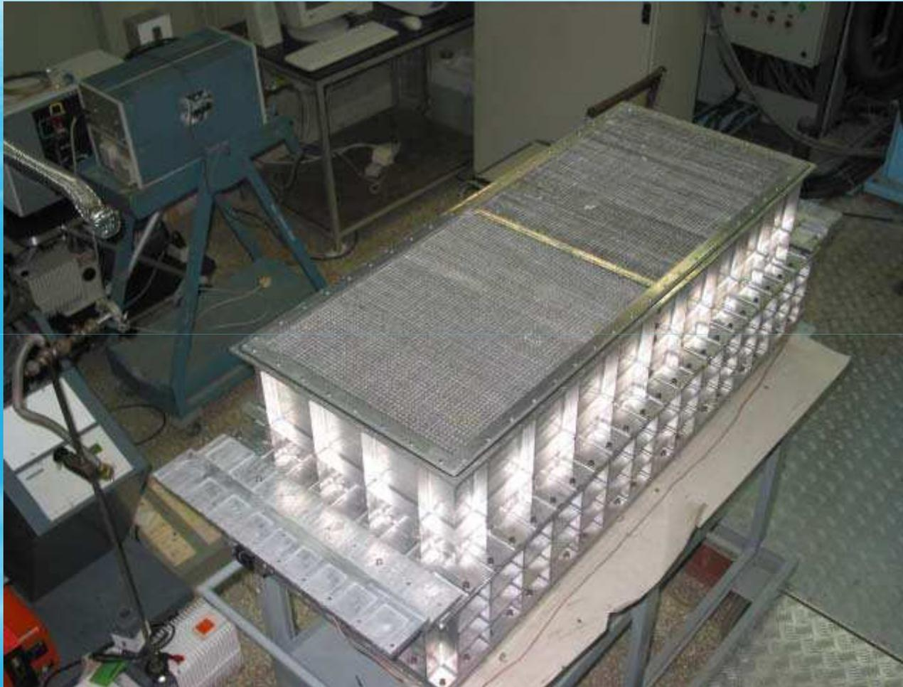
**LAXPC unit with FOV Collimator installed
