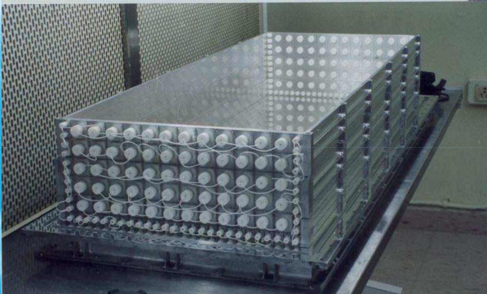
**LAXPC X-ray detecting anode assembly with veto layer on 3 sides mounted on the back plate.**
