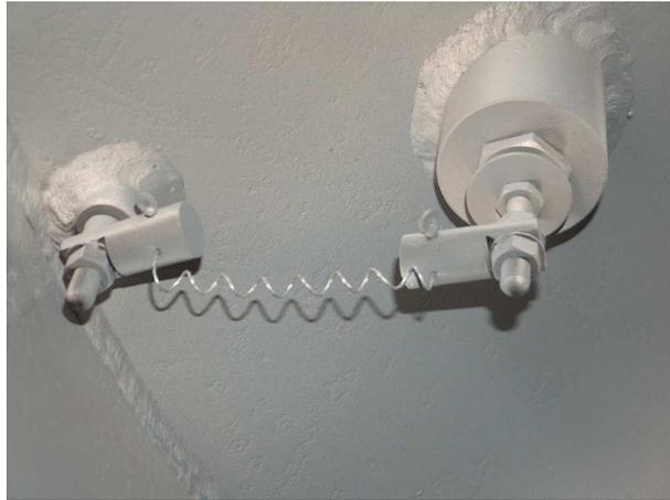
Figure 10: An aluminising coil in the 1m tank
