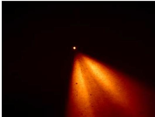
Figure 43: Sodium “guide star” with associated cone caused by Rayleigh scattering.
