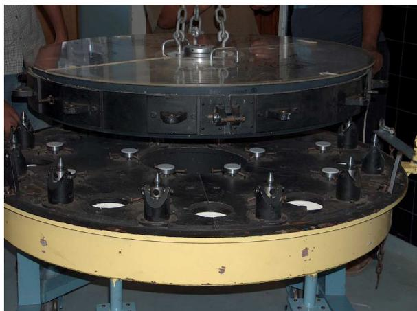
Figure 12: ... and lowered into the mirror cell (note mirror support elements).
