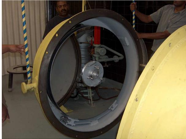
Figure 11: The SAAO 1m mirror being taken out of the aluminising tank ...
