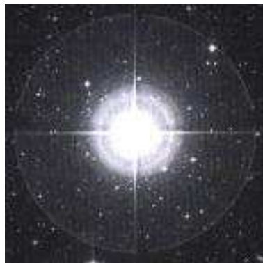
Figure 17: Optical effects from bright images – diffraction and halation.
