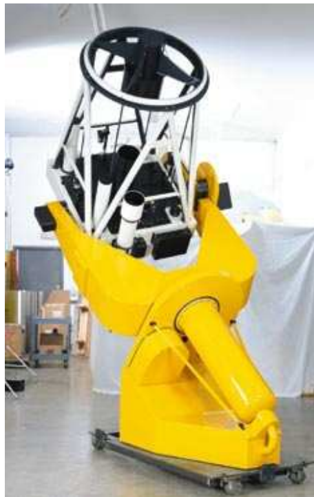
Figure 38: Fork mount telescope. See also the picture of the Anglo-Australian Schmidt telescope in section 4.5
