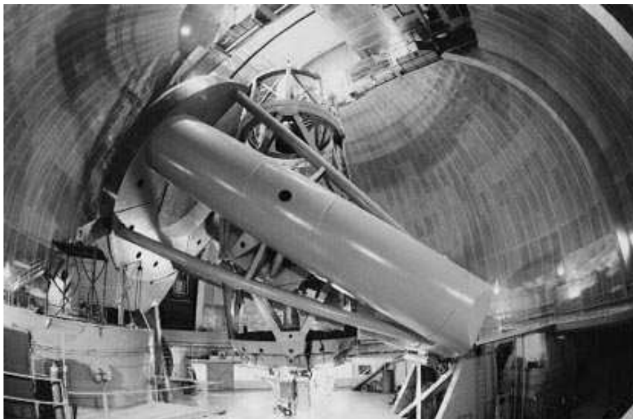
Figure 42: Mt Palomar Observatory 200-inch (5m) telescope. Horseshoe mount – see also the picture of the Anglo-Australian 3.9m telescope in section 4.2.
