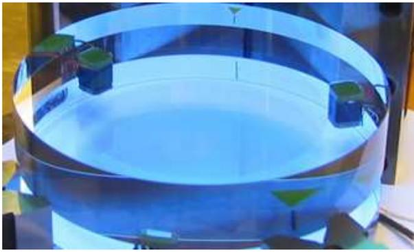
Figure 28: Large (80mm) LightMachinery piezo-tunable Fabry-Pérot interferometer.
