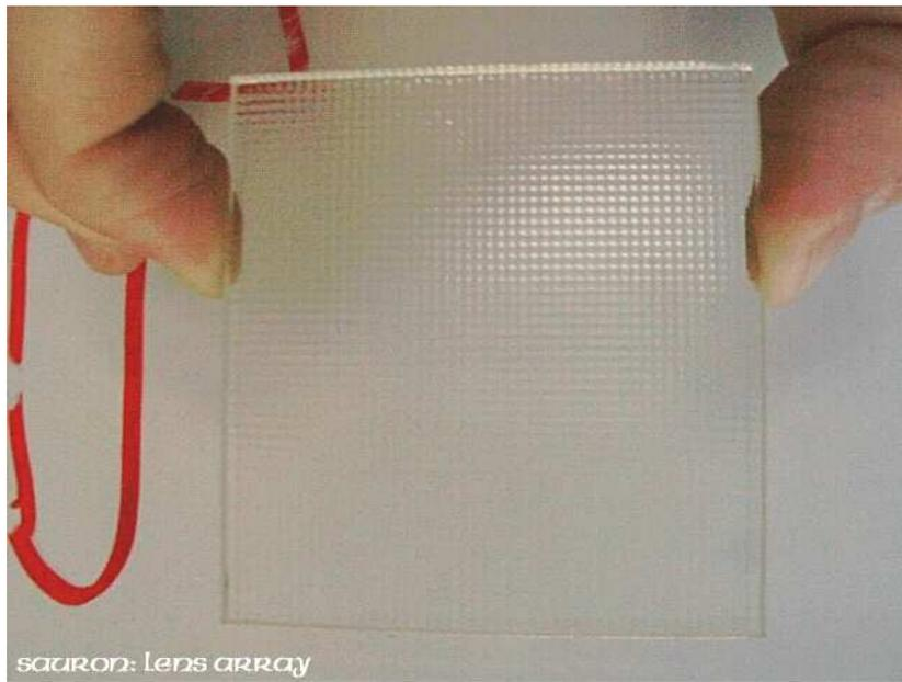
Figure 40: The lenslet array for SAURON – over 1600 square lenslets, each about 1.35mm square. Each lenslet images about  $0.94 \times 0.94$  arcsecs, giving a fully covered field of about  $33 \times 41$  arcsecs – “one eye that sees all”.
