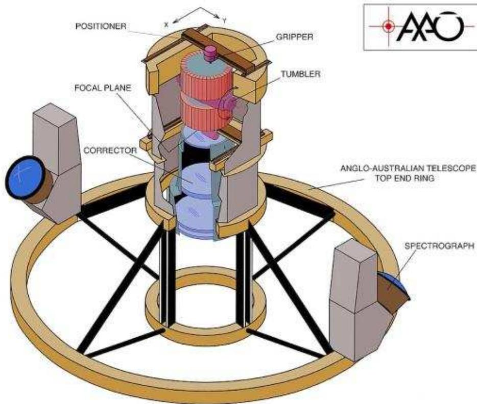
Figure 24: Schematic of the top end of the AAT. This is very smart; since it takes about 30 or 40 minutes to set up each fibre/prism observing field (containing up to 400 fibres) the 2dF has two such systems back-to-back on a “tumbler”. Whilst one field is being observed, the other field is re-positioning.
