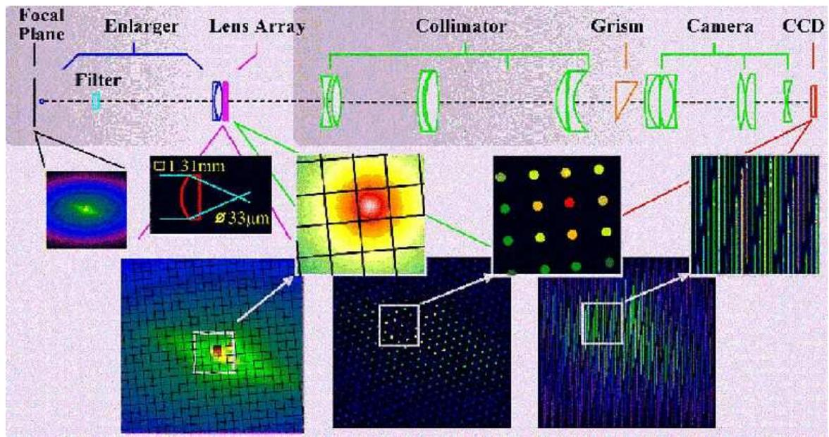
Figure 39: Schematic layout for SAURON – pupil imaging using a lenslet array. The filter selects the wavelength range and the enlarger images the sky on to the lenslet array. The collimated light is dispersed by a grism and a camera images the the spectra to a CCD.
