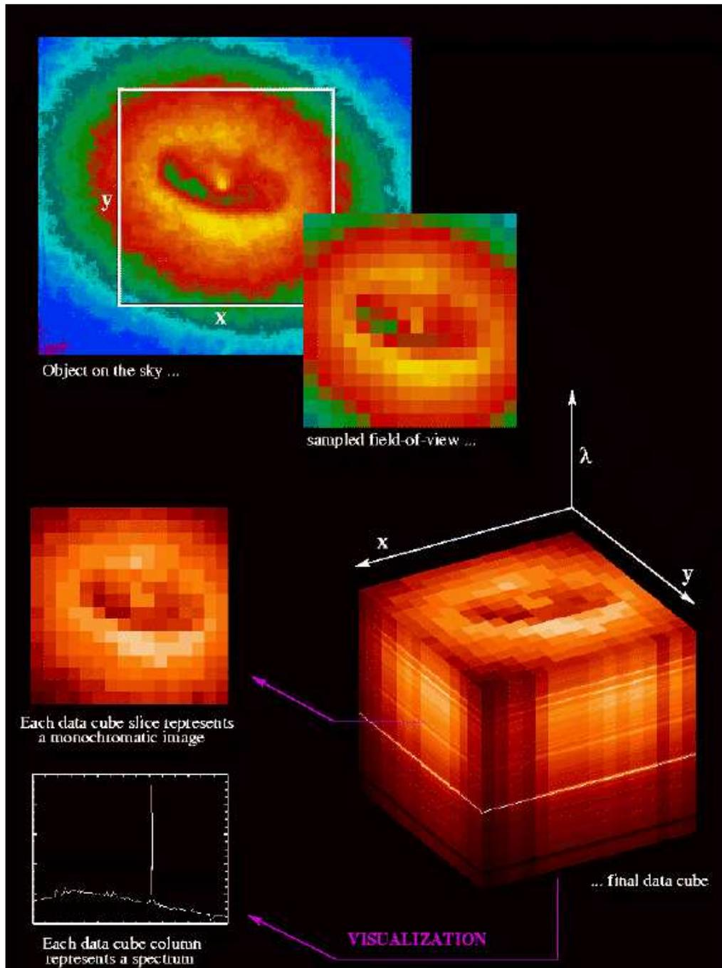
Figure 36: The data cube. A 2-dimensional field (white rectangle) is sampled into discrete spatial elements (which need not be square). These are sometimes called **spaxels** - spatial pixels. The data cube can be sampled “horizontally” to give a monochromatic image of the source (or broader band images by co-adding “slices”) or can be sampled “vertically” to give spectra related to an  $(x, y)$  point.
