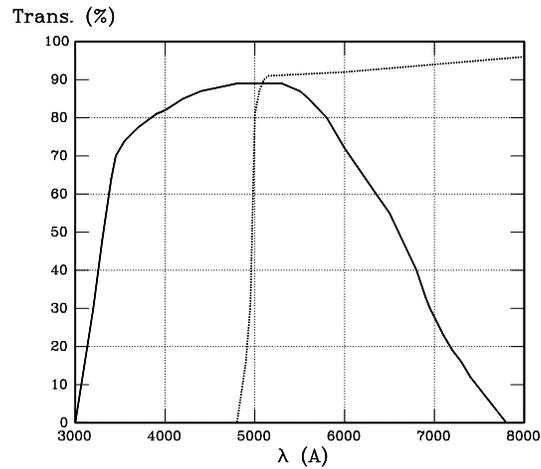
Figure 7: typical “order blocking” filters: solid line BG39; dotted line GG495.
