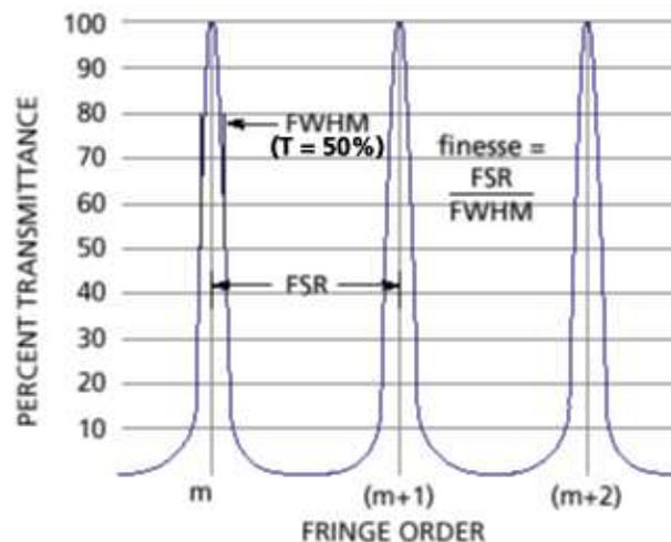
Figure 30: Definition of free spectral range and finesse.
