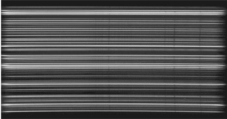
Figure 23: Spectra of  $\sim 100$  stars piped to a single slit.
