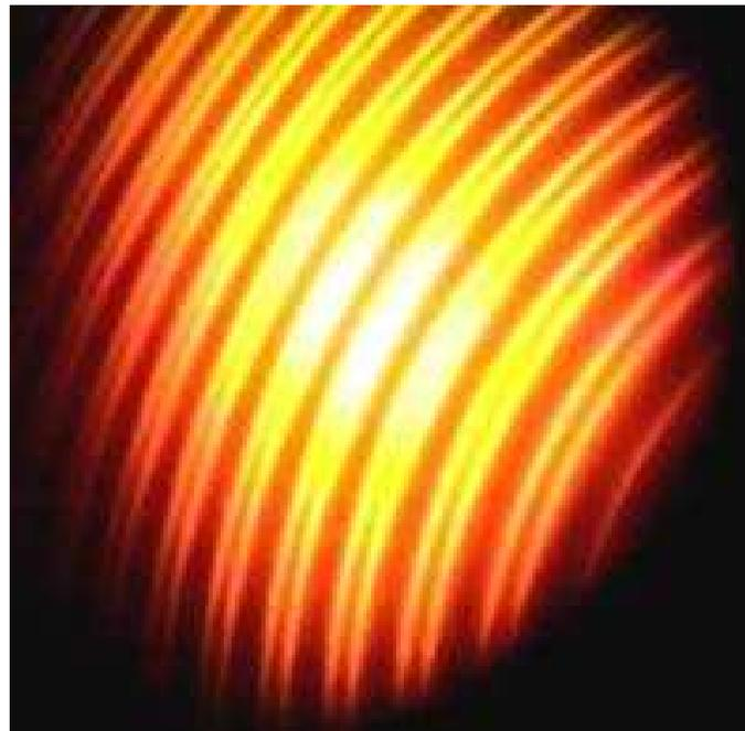
Figure 27: Sodium “D” lines through a Fabry-Perot interferometer.
