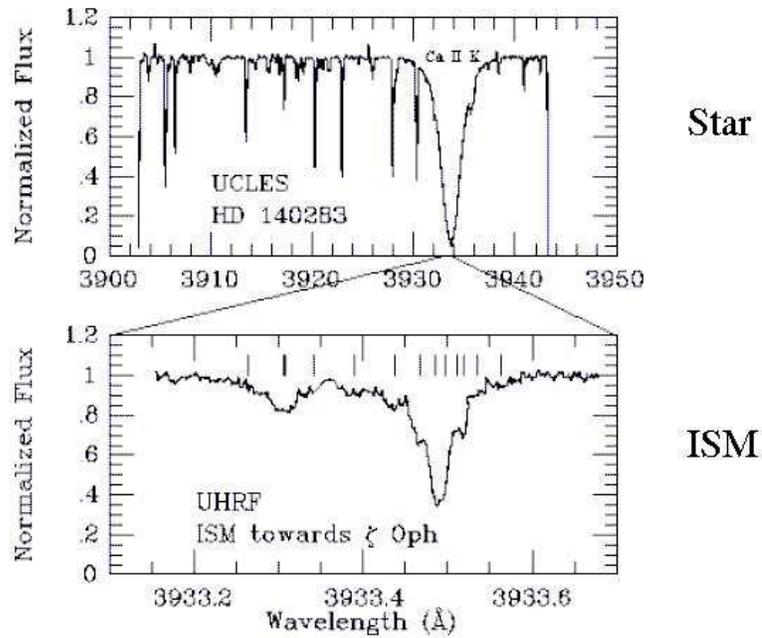
Figure 18: Sample of a single order from an echelle spectrogram.
