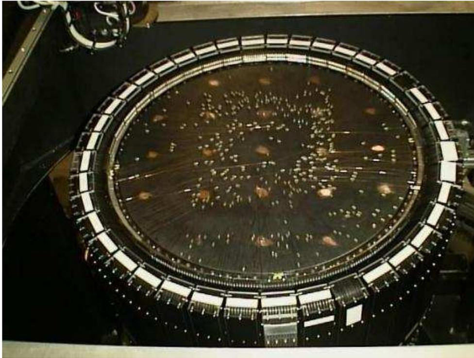
Figure 19: The 2dF fibre system on the AAT. Each speck on the plate is a small "upward looking" prism in a small magnetic holder feeding an optical fibre. A robotic "gripper" takes each prism and places it on a metal plate. The required accuracy is a few tenths of an arcsecond, so accurate astrometry is needed beforehand.
