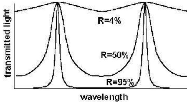
Figure 31: Increase of finesse (resolution) with increasing reflectivity of the Fabry-Pérot plates.
