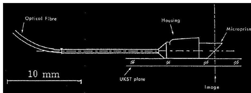
Figure 20: Schematic of a "microprism" assembly from the AAT Schmidt's 6dF.
