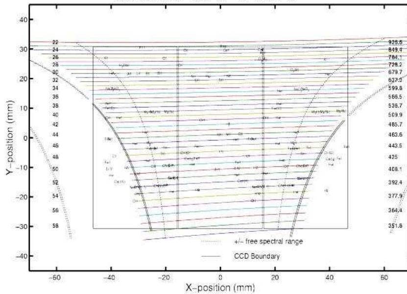
Figure 15: Simulation of the SALT echelle CCDs and order distribution.
