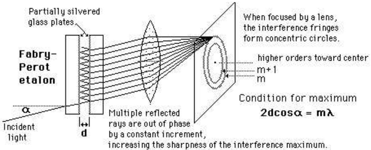
Figure 26: The Fabry-Perot interferometer.
