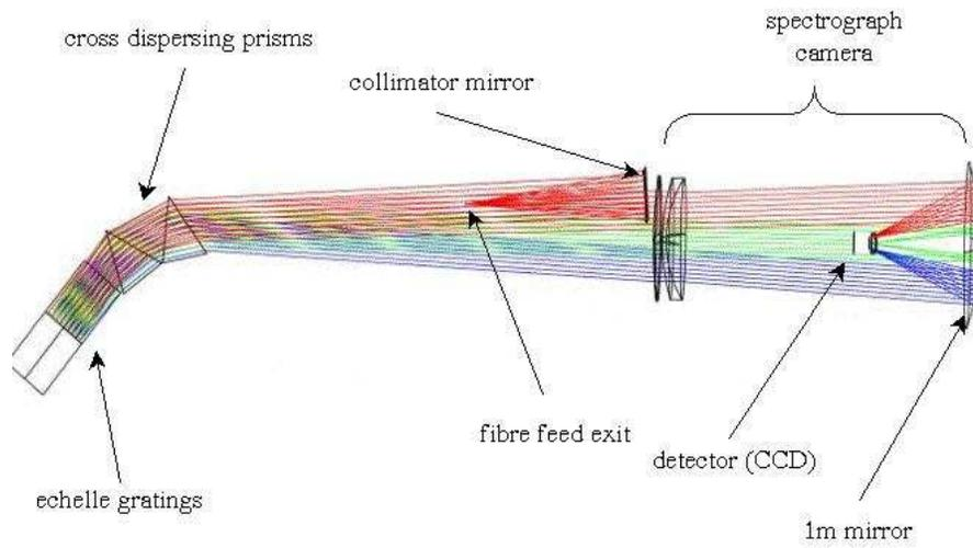
Figure 14: Suggested “double-pass” prism cross-dispersers for the SALT Hi-Res spectrograph.
