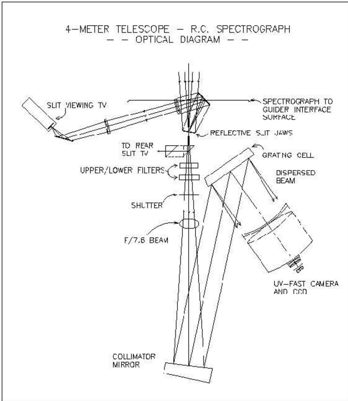
Figure 6: Schematic of the KPNO Cassegrain spectrograph
