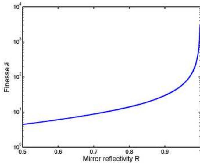
Figure 32: Increase of finesse (resolution) with increasing reflectivity of the Fabry-Pérot plates.
