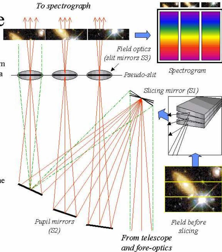
Figure 37: Durham University (UK) designed image slicer.
