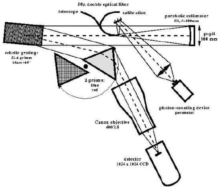
Figure 12: Schematic of the “MUSICOS” spectrograph a copy of which is used on the SAAO 1.9m. The cross-disperser is a prism. Either of two prisms can be used; one optimised for the blue and one for the red.
