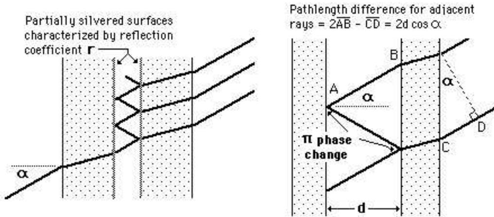
Figure 25: The basis for a Fabry-Pérot interferometer (note: the angle  $\alpha$  is exaggerated for clarity).
