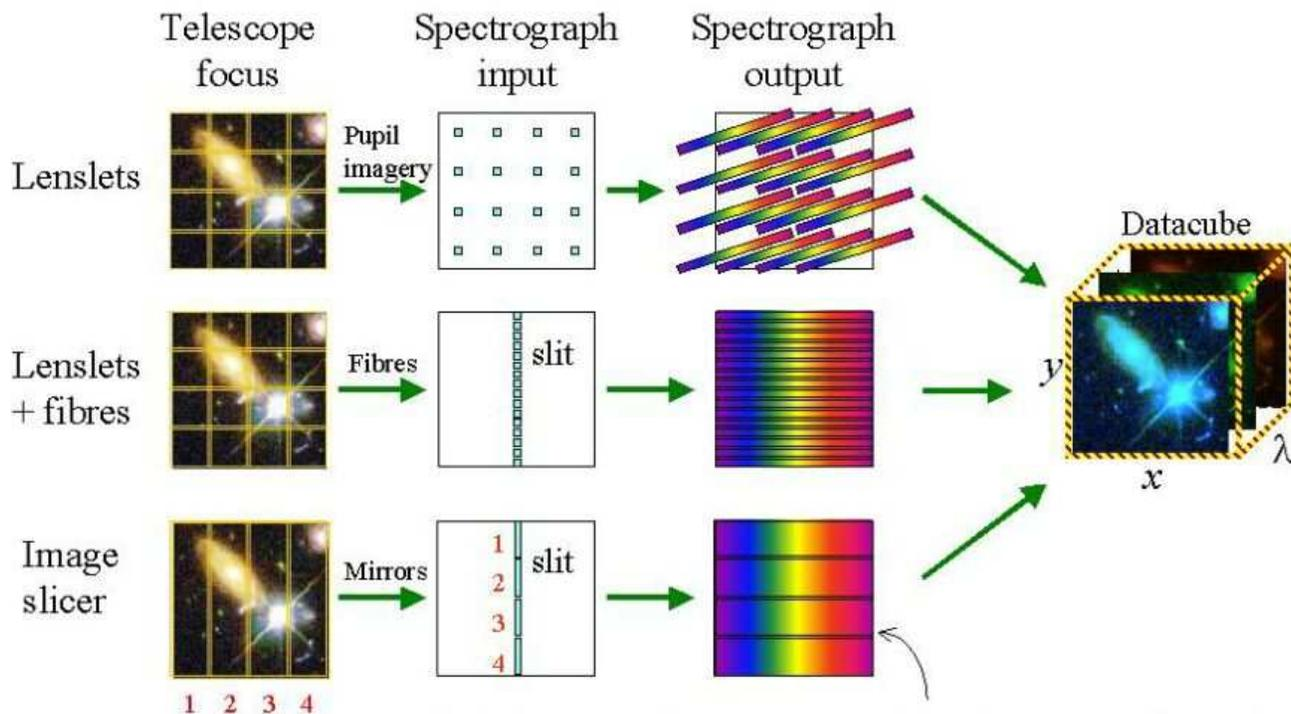
Figure 35: Basic ideas of integral field spectroscopy.
