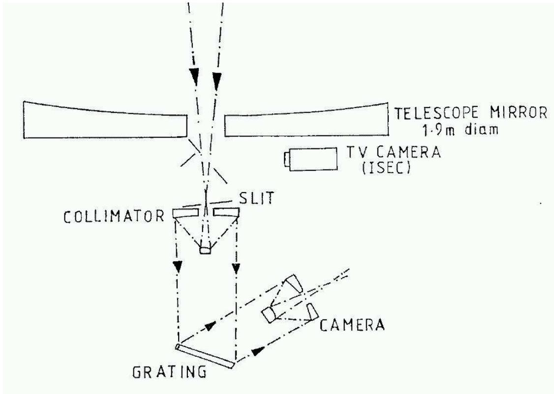
Figure 5: Schematic of the Cassegrain spectrograph used on the SAAO 1.9m
