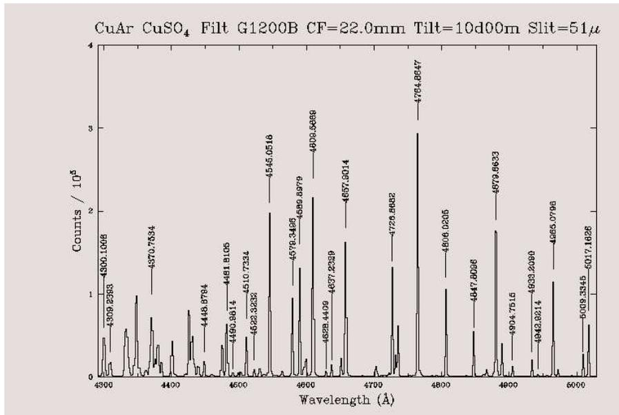
Figure 10: Small range of frequencies from a Copper-Argon arc lamp.
