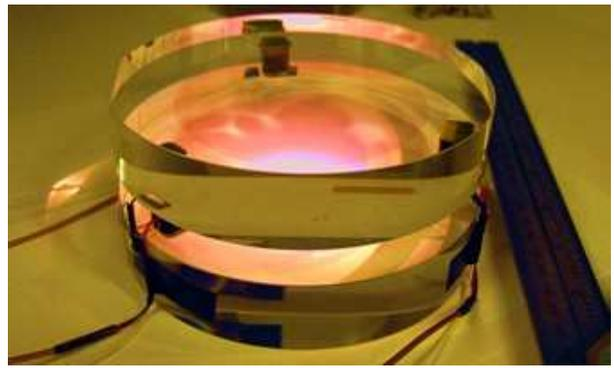
Figure 29: LightMachinery piezo-tunable Fabry-Pérot interferometer.
