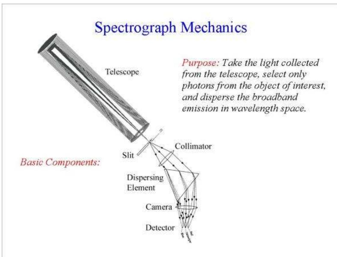
Figure 1: Schematic of a conventional (typically Cassegrain focus) slit spectrograph.
