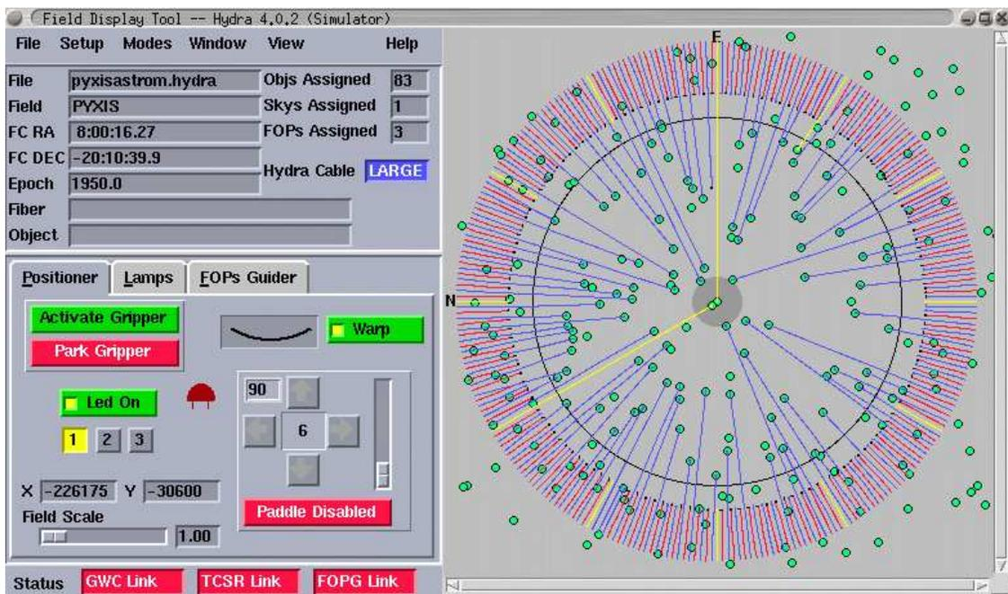
Figure 22: NOAO “Hydra” set-up software interface, set for stars in the Pyxis globular cluster. The yellow-coded fibres pick up “fiducial” bright stars for guiding.
