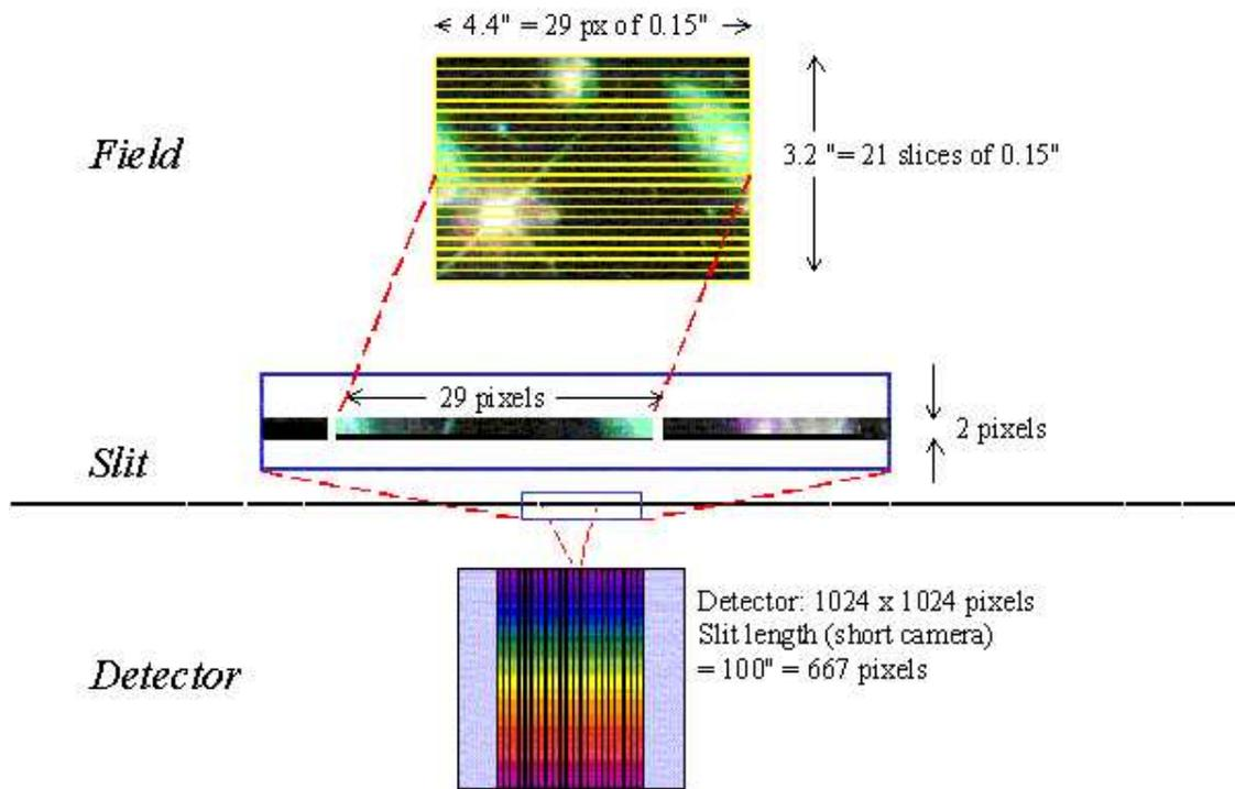
Figure 38: Schematic for the GEMINI Near Infrared spectrograph (GNIRS) – an image slicer system.
