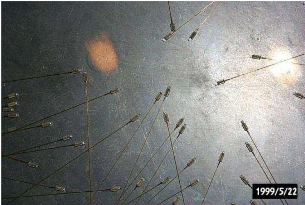
Figure 21: Close up of the 2dF fibre feeds on the metal plate.
