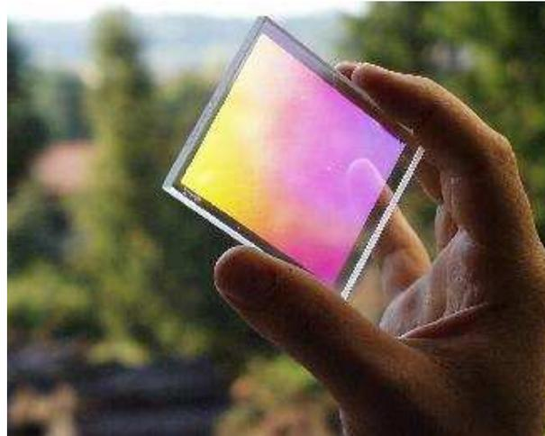
Figure 30: A Volume Phase Holographic Grating.
