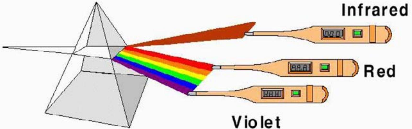
Fig. 1: Herschel used a prism and thermometers in his experiment that eventually led to the discovery of the infrared region of the electromagnetic spectrum.
