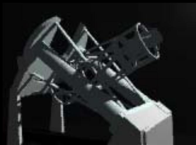
**Light Path** — Keck Telescope diagram shows the path of incoming starlight (1), first on its way to the primary mirror; reflected off the primary, toward the secondary mirror (2); bouncing off the secondary, back down toward the tertiary mirror (3); and finally reflected either off the tertiary mirror to an instrument at the Nasmyth focus (4), or to the Cassegrain focus (5) beneath the primary mirror.
