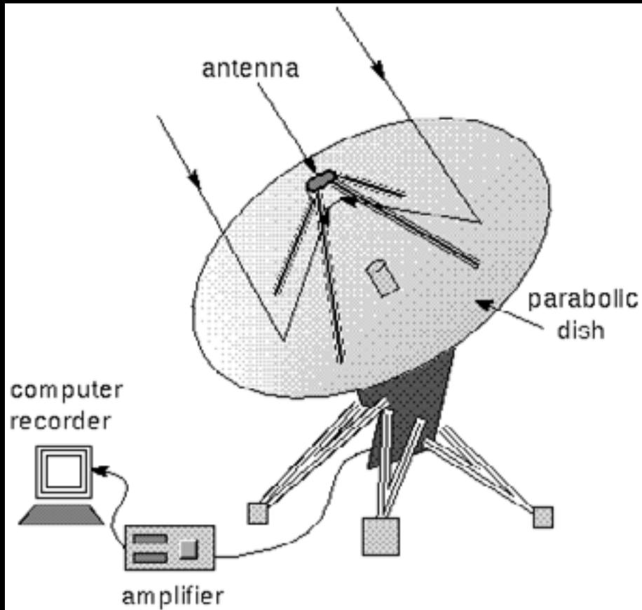
A radio telescope reflects radio waves to a focus at the antenna. Because radio wavelengths are very large, the radio dish must be very large.
