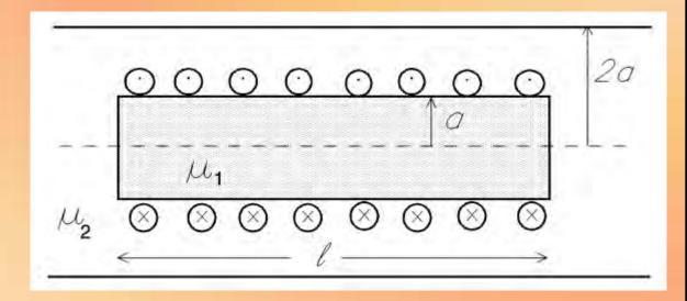
**Q.3.** Solution: (b) Apply Ampere's circuital law to the anticlockwise rectangular path shown:  $\oint \vec{H} \cdot d\vec{l} = n I dl$  (*n* turns per unit length, *n dl* times current *I* in length *dl* )
