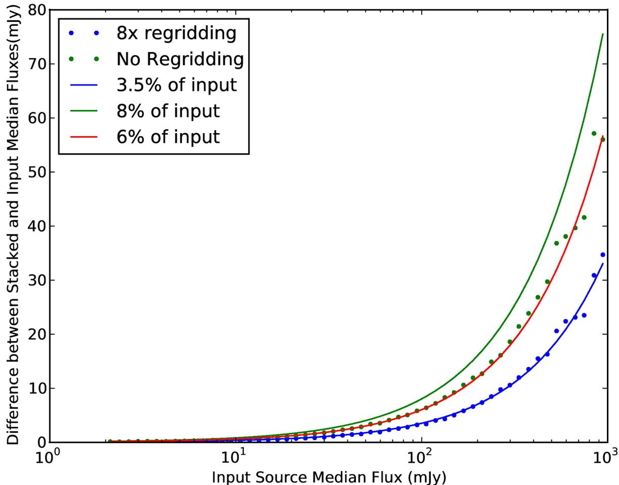
Alignment to nearest pixel introduces a downward systematic error depending on sampling.
