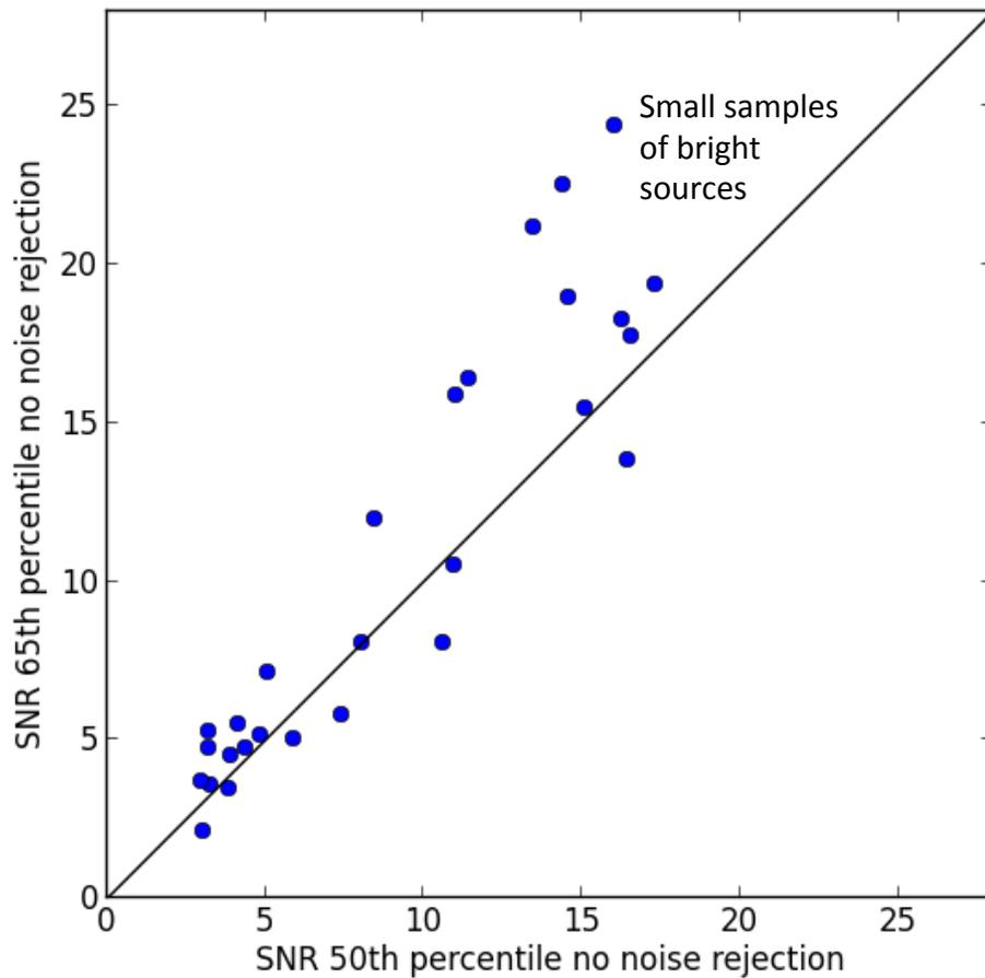
Measured signal-to-noise ratio for polarized intensity in stacking ATLAS DR3 fields, median stacking versus 65<sup>th</sup> percentile.
