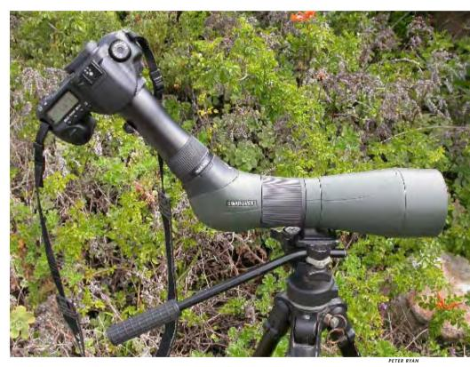
Attaching a digital SLR to a telescope may seem like a perfect solution to many of the problems of digiscoping, because you can see through the viewfinder. However, image quality doesn't compare with that produced by a compact digital camera.
