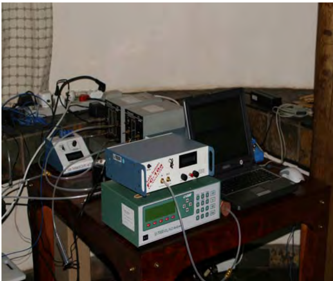
A portable respirometry system used to measure metabolic rates of wild birds in the field. Photo: Andrew McKechnie.
