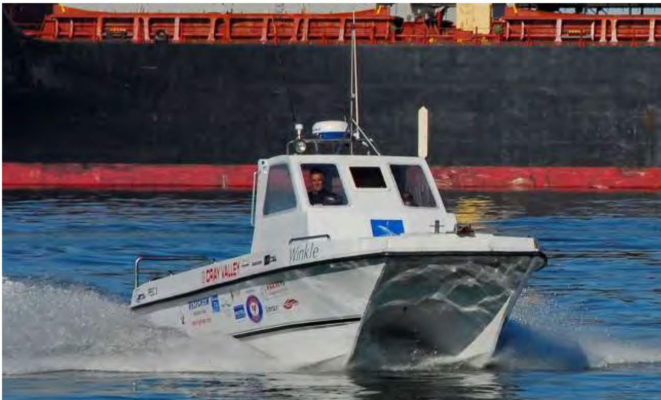
The newly launched research boat 'Winkle' with a state-of-the-art, multi-scan sonar system which can estimate the abundance and movements of the fish prey of the Endangered African Penguin. (Photo: Gary Davis)
