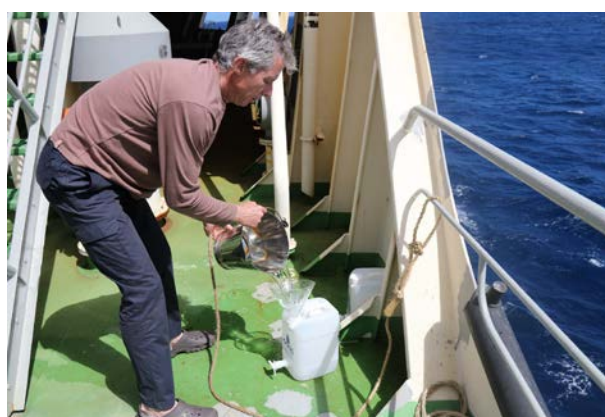
Peter Ryan sampling surface waters for microplastics from the bow of the Akademik Tryoshnikov during ACE, using a stainless steel bucket and natural-fibre rope (Photo: Fabrice Le Bouard).
