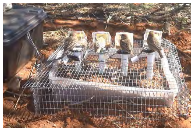
A new system to collect social associations uses RFID readers to read the PIT-tag numbers when the birds come to the feeders (Photo André Ferreira).
