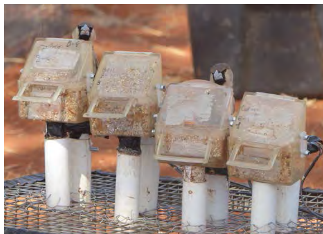
Feeding stations equipped with RFID antennas are now operating at five colonies to automatically collect data on associations between individuals (Photo Cécile Vansteenbergh).
