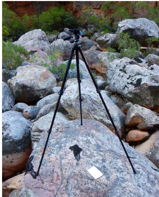
Figure 3. Tripod positioned on rocky platform. Tripod legs are set such that tripod head is as level as possible.
